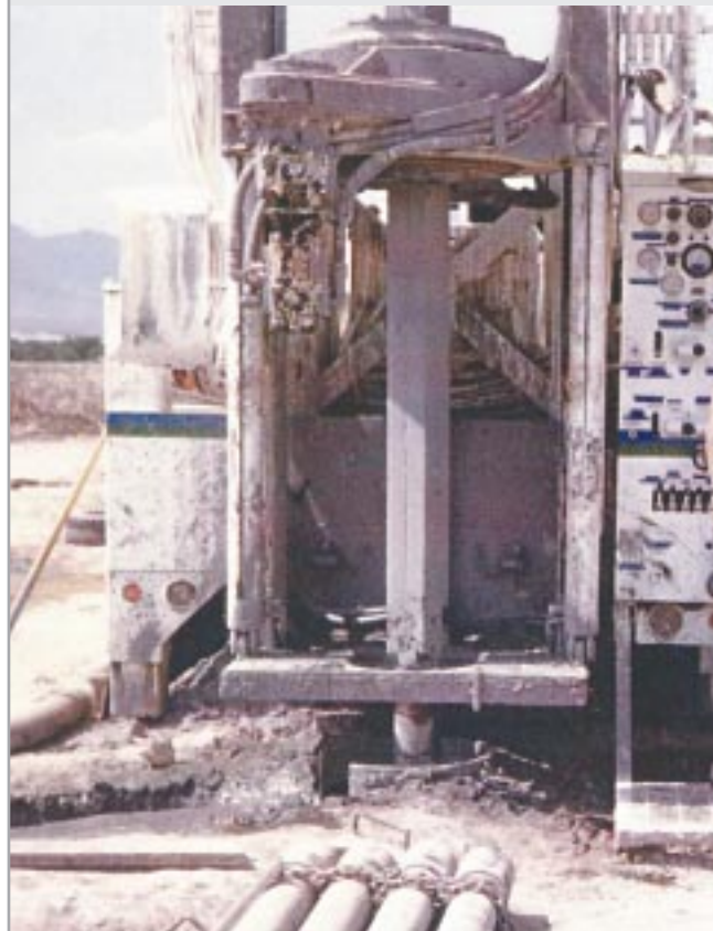
Dual Rotary rig in kelly bar drilling application.
