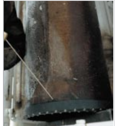
A carbide-studded casing shoe is welded to the bottom of the first casing joint.
