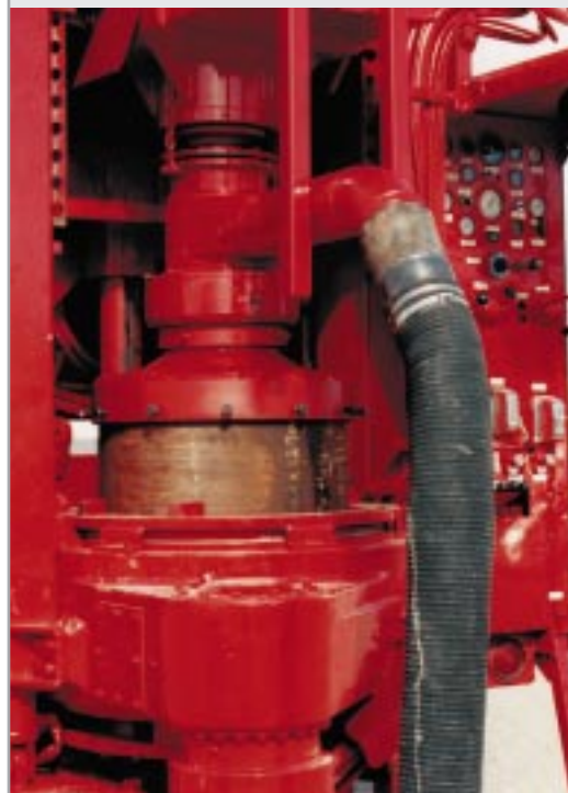
Standard discharge swivel sizes are 10" (254 mm), 16" (406 mm) and 24" (610 mm) and can accommodate 3 1/2" (89 mm) to 18" (457 mm) diameter drill pipe. Discharge swivel adapters allow the swivel to be fitted to other casing sizes.
