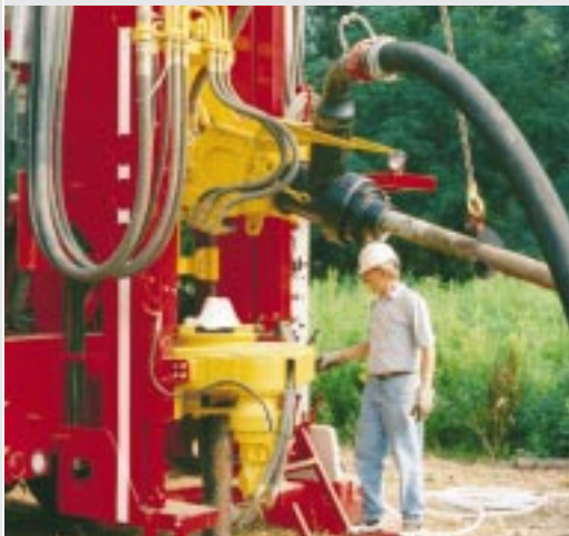
Standard tilting top-drive enables safe handling of drill pipe and casing.
