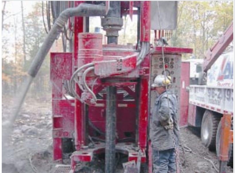
Cuttings are typically evacuated using air from the on-board compressor. The DR can also be setup for mud or reverse-flooded applications. Note how the cuttings are diverted through the discharge swivel. A longer discharge hose can be added to direct cuttings to a designated dumping point, container, or optional sampling cyclone.
