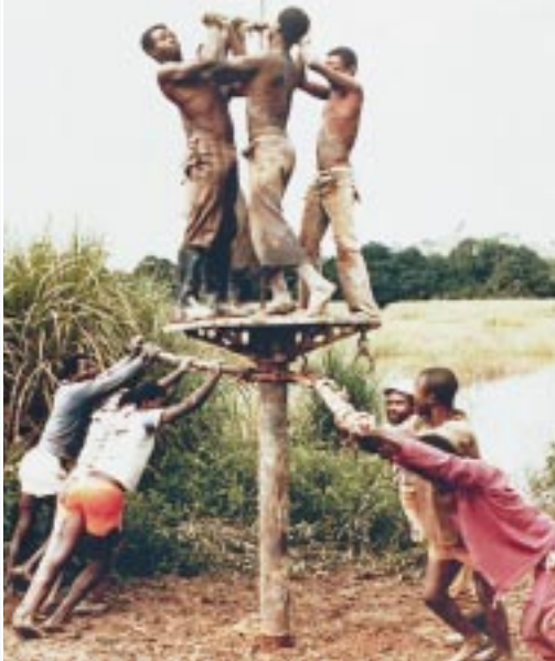
Manual representation of the forces at work when Dual Rotary Drilling, including pulldown and rotation for both the drill string and casing
